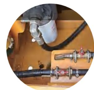
Engine compartment volume is increased by 20%, and water drain valve and diesel oil check valve are added
