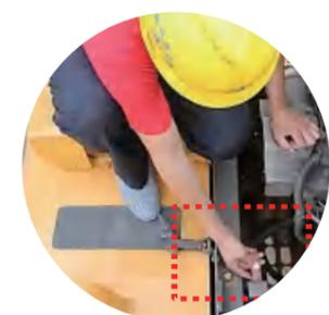
Easy to inspect engine oil; pump oil by one push after engine goes off abnormally
