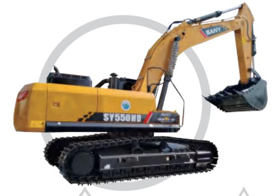
Bucket rod adopts bottom plate reinforcing bars and forging front support etc. As compared with competitor brands, the stress on main loading point is **30% lower**, and the service life is **30% higher** under mining conditions.
