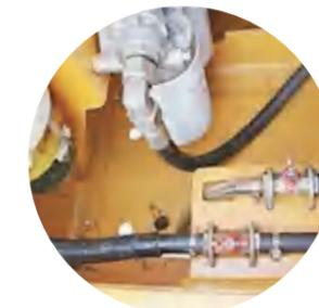
Water drain valve and check valve of fuel tank
