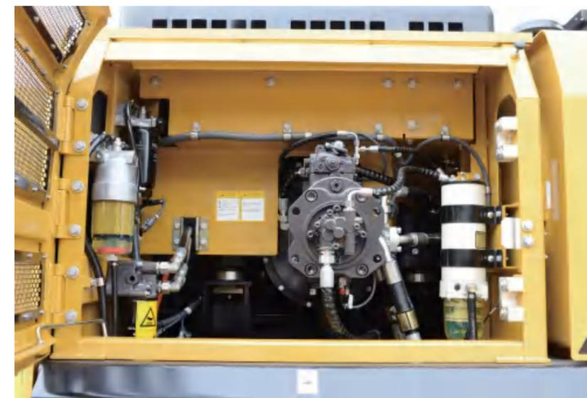
Large-capacity multi-stage filter system
