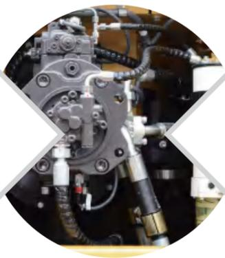
Kawasaki 160CC dual-ratio positive-flow main pump takes full advantage of the flow and realizes demand equal to supply. As compared with negative flow system, it reduces the loss of neutral-position return, and meanwhile response speed is higher and capacity loss is reduced
